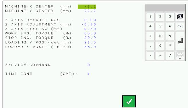
The parameter of the engraving depth is **Z AXIS ADJUSTMENT (mm) : -0.70**
